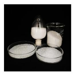
White fused alumina is made of high-purity low-sodium alumina powder by melting at the high temperature, cooling crystallization, and then crushing. The white fused alumina grit is under strict controlling to keep the grain size distribution and the consistent appearance.
