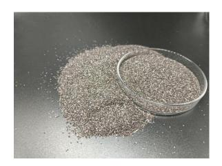
Brown fused alumina is a tough, hard material (Mohs hardness 9) with high strength, excellent wear and corrosion resistance and good thermal conductivity. It is produced by controlled melting of calcined bauxite in an electric arc furnace. Furthermore, BFA is the perfect media for removing rust, mill scale, and surface contamination due to its high bulk density and hardness. The consistent particle size allows for a uniform surface finish and coverage.
